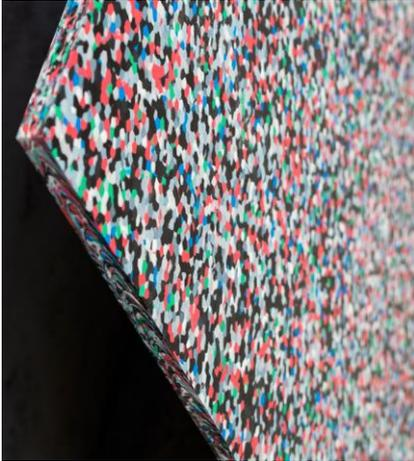
**The product in the Building & Construction category is called Voronj. It is a panel that varies in size and thickness (0.4 to 4 cm) made by the Italian company Plastiz.** The panel is entirely made of a particular grade of HDPE branded Sertene<sup>®</sup> from post-consumer mechanical recycling and can be used for different indoor and outdoor applications, both decorative (garden objects, complements, etc.) and functional (insulation panels, decoration of interiors and exteriors).
